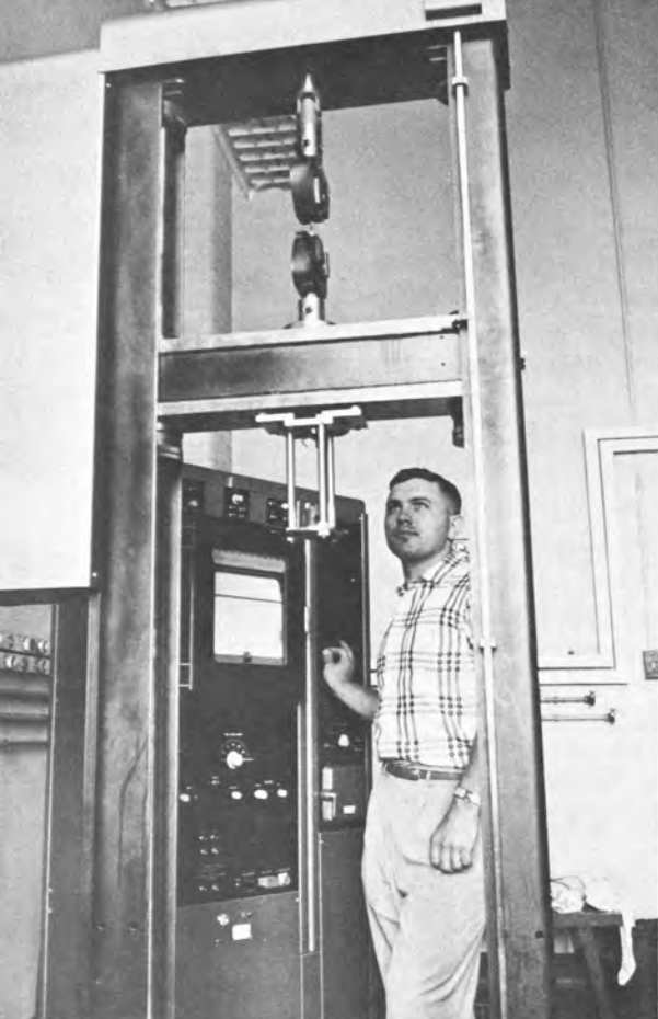
A Jr. Research Metals Engineer uses the Instron testing machine to strain zone-melted, high purity iron prior to growing a single crystal.
